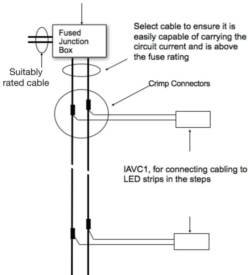
For long cable runs it is recommended that power is fed to both ends of the wiring
